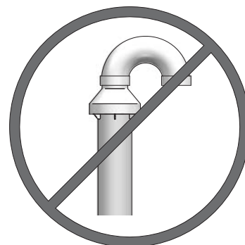
Figure 5-5 Do Not Install U-Bend to Rain Cap
